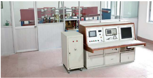
Impulse Current Generator
