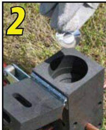
Install steel disk in the mold.
